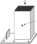
Secure Post to Guardrail with 3/8" Lag Bolt
