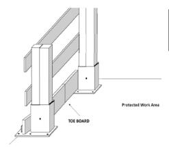
Mid Rails and Top Rail / Hand Rails should be located and secured to Post according to OSHA Guidelines.
